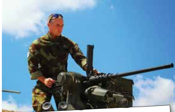
Kongsberg M151 Protector RWS (remote weapon station) mounted on a Mowag Piranha in UNIFIL. Note the bottom mirror-like lens belonging to its thermal imager.
