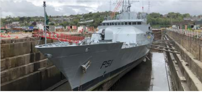
Each keel block and each supporting beam are placed according to a well laid plan.
