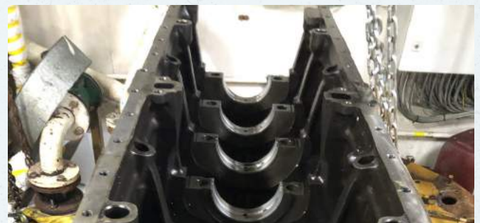
A generator is maintained according to its running hours. Here one is undergoing a complete rebuild; the only part remaining in place is its crankcase.
