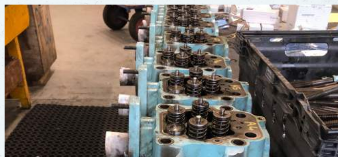
A row of engine cylinder heads awaiting individual overhaul in a marine engineering workshop.
