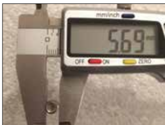
● Figure 3: SS109 Bullet Base and Pre-Fire Diameter. Note the exposed core.
