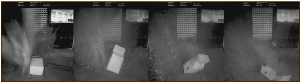
Figure 1: A four-picture sequence showing an experimental setup in which a model vehicle weighing 150 kg is subjected to blast loading from a buried 'IED'. Note that the vehicle undergoes severe acceleration and is thrown upside-down. 11
