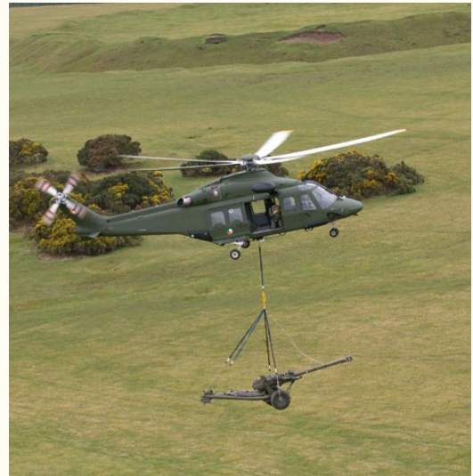
The new AW 139 helicopter airlifts a 105mm Light Gun during a training exercise.
